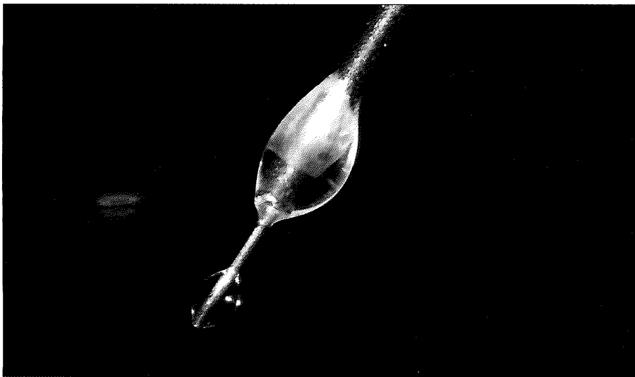
The newer cannula has a rigid tip, an overall diameter of 150 \mu\text{m} , an internal diameter of 38 \mu\text{m} and an increased length of 2 mm.
